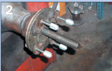
1. Hendrix Wire Wheel has adapters for virtually any type of British wire wheel. 2. Wheels or drums can be mounted to the balancer using lug nuts to perfectly mimic how they will behave on the car. 3. Shaving the high points off tires is key to getting the shake out. 4. Hendrix Wire Wheel has a European-style tire mounter that won’t bend the spokes on a wire wheel.
