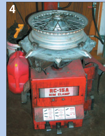
1. Hendrix Wire Wheel has adapters for virtually any type of British wire wheel. 2. Wheels or drums can be mounted to the balancer using lug nuts to perfectly mimic how they will behave on the car. 3. Shaving the high points off tires is key to getting the shake out. 4. Hendrix Wire Wheel has a European-style tire mounter that won’t bend the spokes on a wire wheel.
